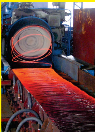
Wire Rod Rolling Mills
