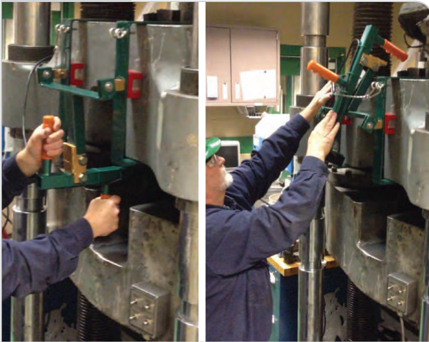
Finished device in use: in active position (left) and storage position (right).
