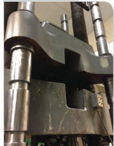
Vertical-style 600-kN tensile testing machine.
