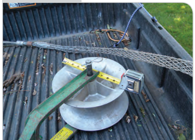
View of pulley and “Chinese finger” in truck bed.
