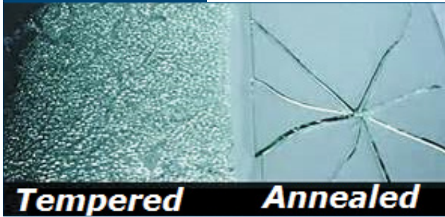
Break patterns in tempered versus annealed glass.
