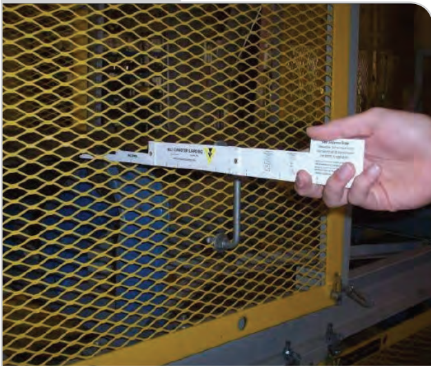
A safety gauge can measure distance to a pinch point.
