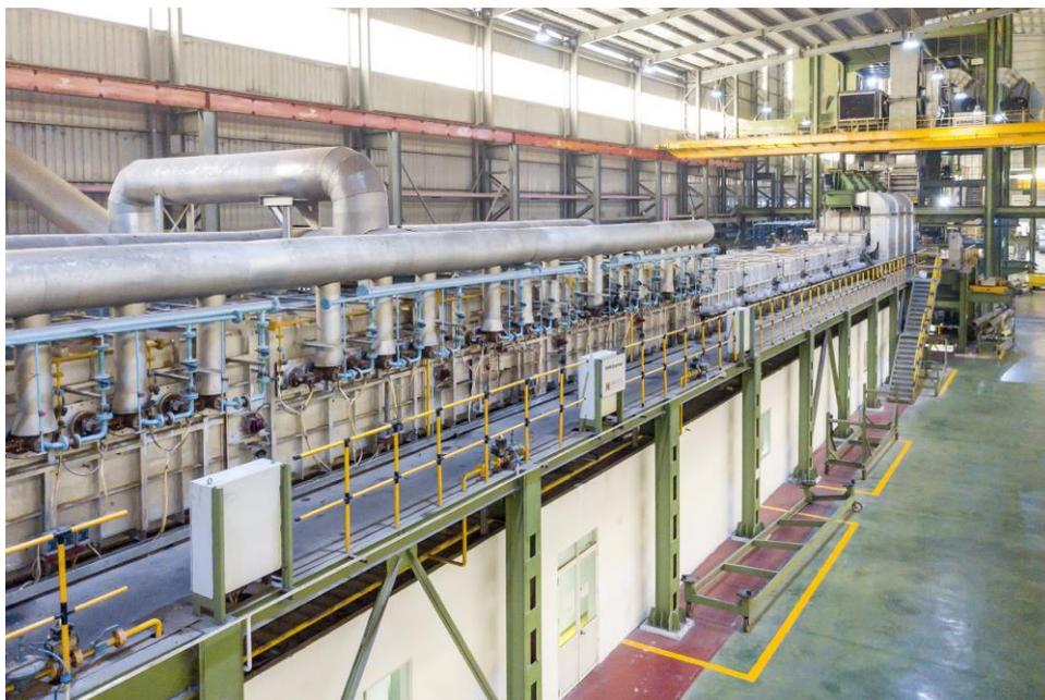
The new line will enable Ruifeng to coat 350,000 tons per year of cold strip for the construction and home appliances industries. The layer to be applied will be aluminum-zinc or zinc.
