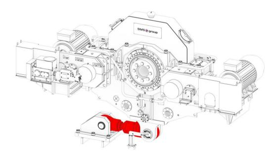
Converter tilt drive with SMS group torque retainer.
