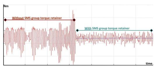
Vibrations of the AOD converter measured over time. Left: without torque retainer, right: with SMS group torque retainer.
