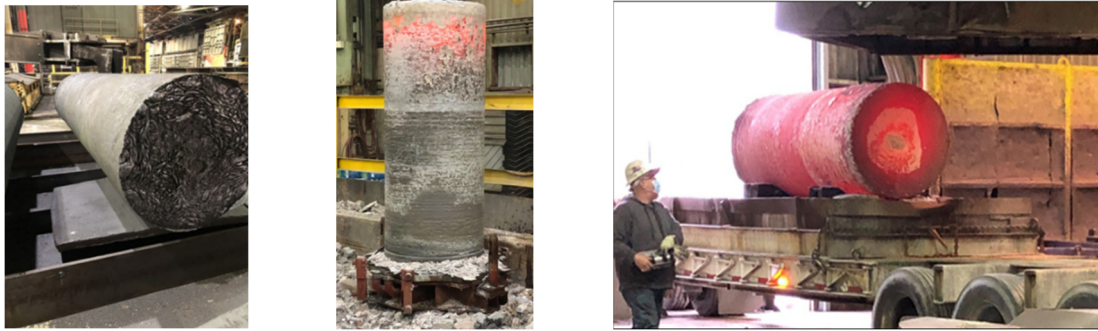
Figure 2. a) As-cast VIM electrode, b) ESR Ingot after stripping, c) Equilibrated ingot delivered for forging.
