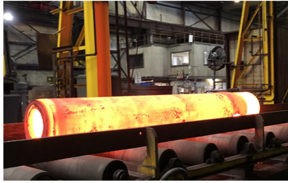
Figure 11. a) Billet ready for blocking, b) As-extruded pipe.
