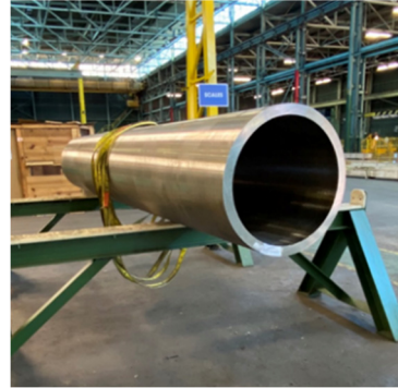
Figure 12. a) 22-inch OD x 4-inch W header pipe, b) 28-inch x 2-inch W reheater pipe.
