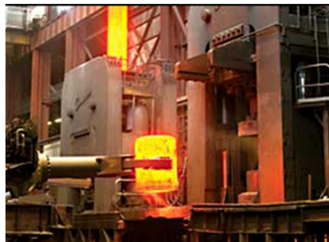
Figure 9. Wyman-Gordon Presses, Left: 35KT extrusion press; Right: 14KT blocking and piercing press.
