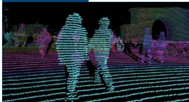
Audi's lidar showing pedestrians. 4
