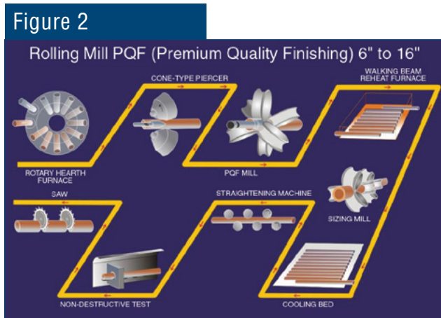
Rolling mill's production flow at VSB Jeceaba.
