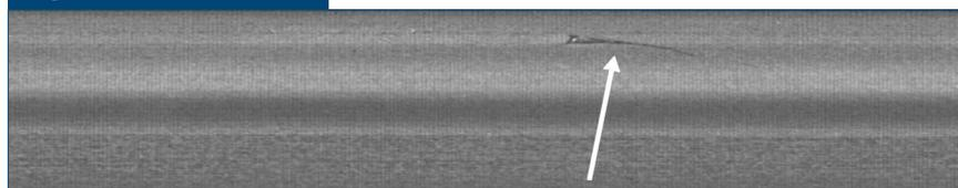
A typical roller crack defect.
