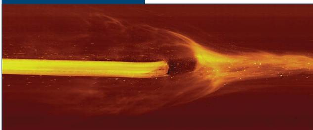
Wire rod nose during hot rolling process at 99 m/second.
