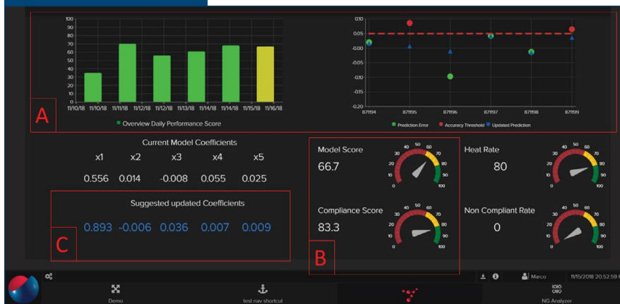
Model Control dashboard for C level prediction in the argon oxygen decarburization process.
