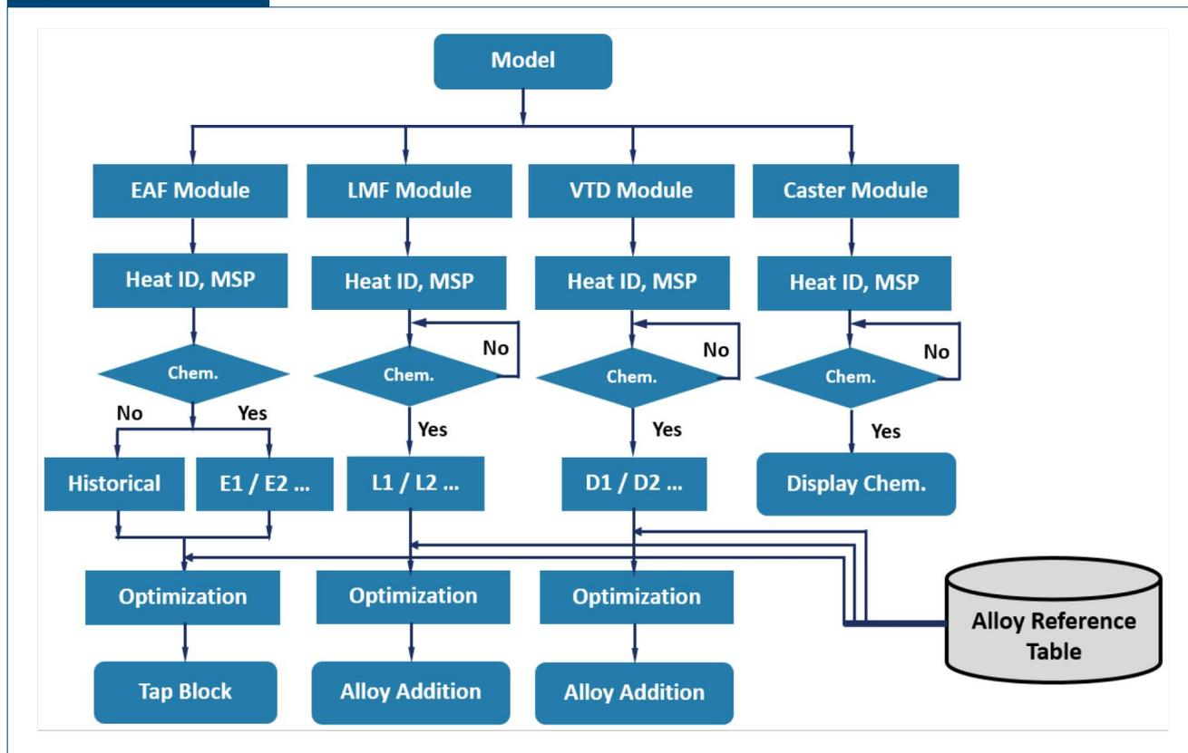
Alloy addition model structure (E1/E2, L1/L2, and D1/D2 represent the chemistry sample identification at the electric arc furnace (EAF), ladle metallurgy furnace (LMF) and vacuum tank degasser (VTD)).
