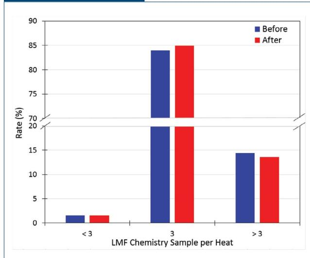
Number of chemistry tests per heat at the LMF.
