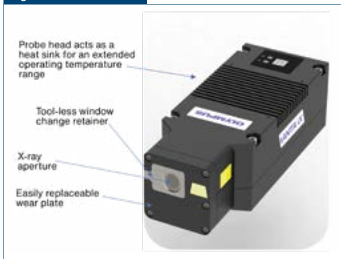
The external envelope features of the Vanta iX analyzer.
