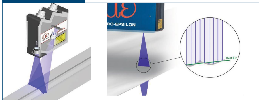
Laser line sensor and value from best-fit line principle.
