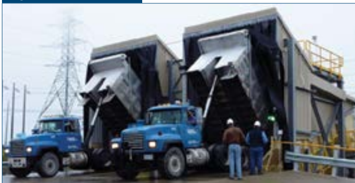
Enclosed and dust-free fuel unloading of materials from road truck. Source: AUMUND Group.
