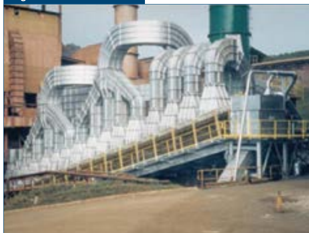
Enclosed and dust-free conveying and cooling of iron pellets. Source: AUMUND Group.
