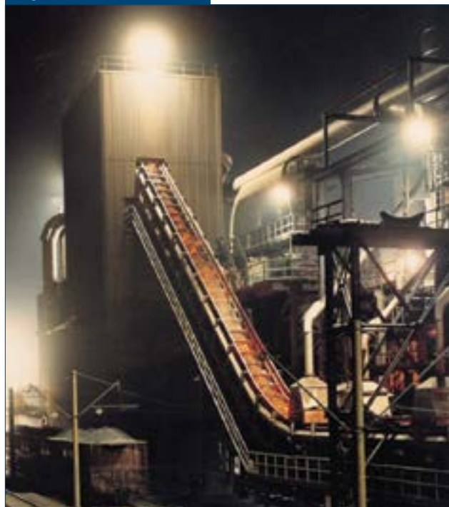
Installed hot sinter conveyor. Source: AUMUND Group.
