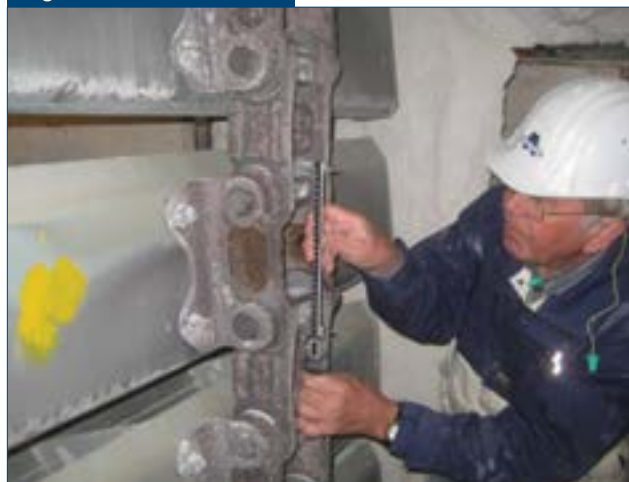
Inspecting chain elongation to ensure clearances are maintained inside equipment to avoid metal to metal wear and contact. Source: AUMUND Group.
