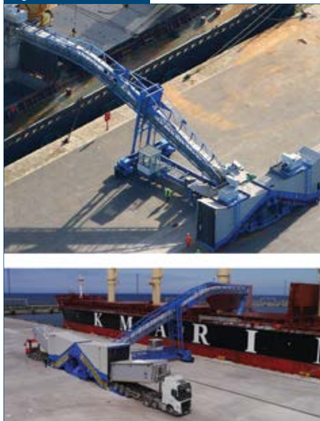
Enclosed and dust-free material loading at port facilities. Source: AUMUND Group.
