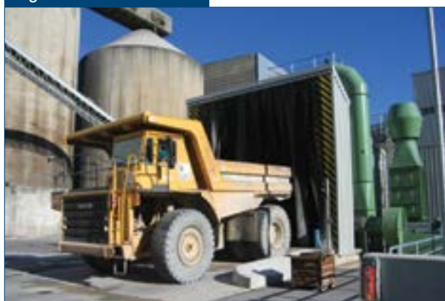
Enclosed and dust-free unloading of materials from run of mine truck. Source: AUMUND Group.
