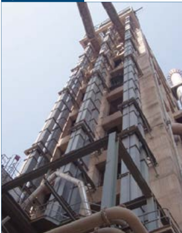
Example of modern bucket elevator transfer height. Source: AUMUND Group.
