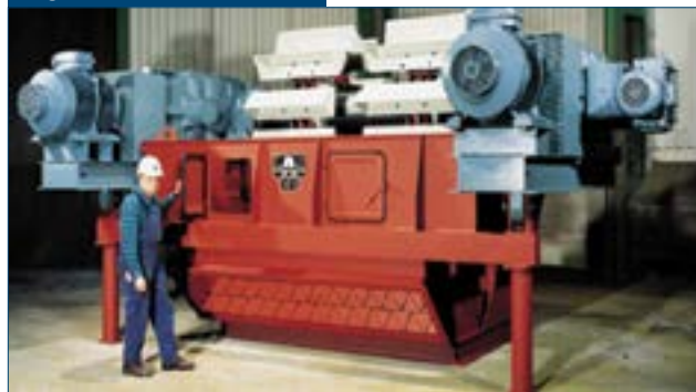
Modern bulk material bucket elevator drive example. Source: AUMUND Group.
