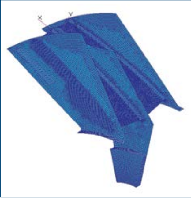
Impeller finite element model for static stress analysis.
