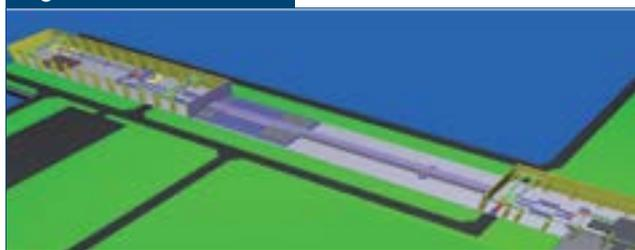
Layout of high-speed coil car system with yard management system.
