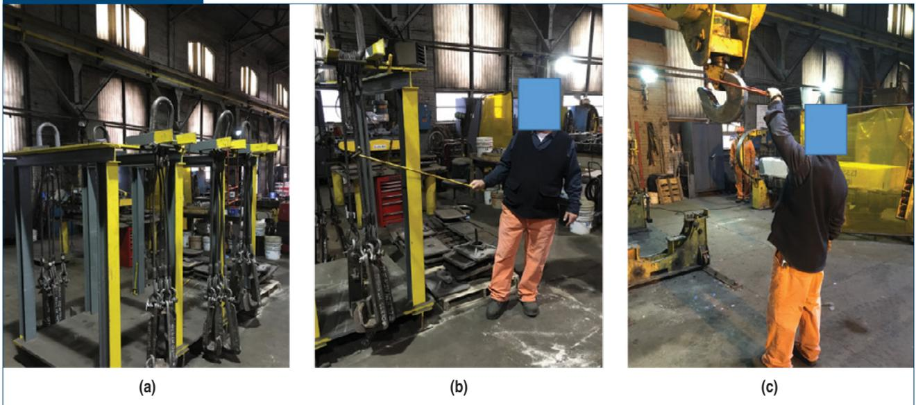
Vertical shelf to hang crane hooks and chains (a), and special tools to guide the chains (b) and to open the crane hook (c).
