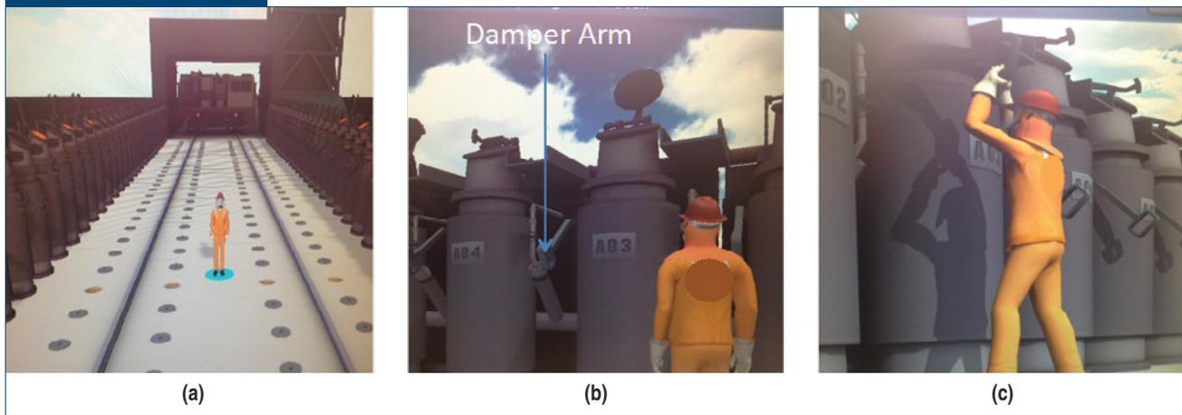
An overview of coke oven batteries (a), damper arms (b) and worker's arm posture when exerting high force on stiff/stuck damper arms (c).
