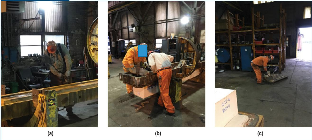
Working with the manual vibrating gun (a), and awkward postures observed at the site (b and c).
