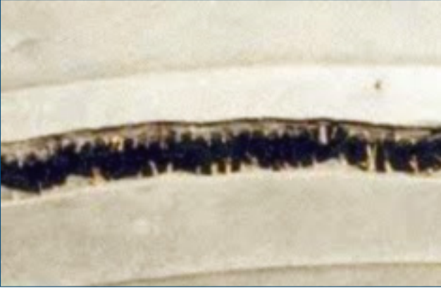
Detailed photo of a zipper rupture.
