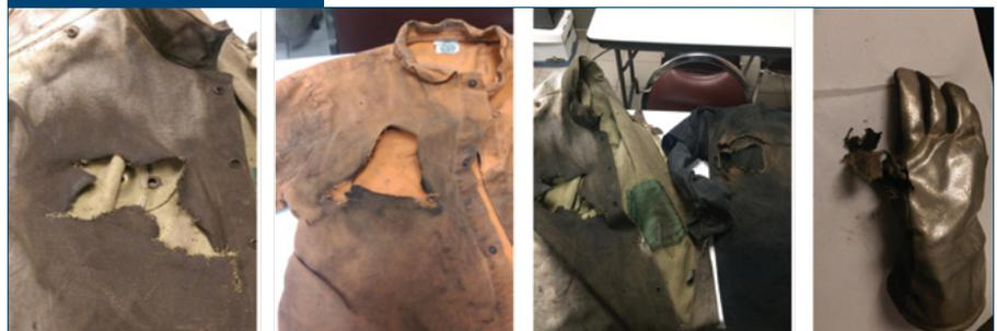
*Damage to personal protective equipment (PPE) as a result of Brad's oxygen lance incident.*
