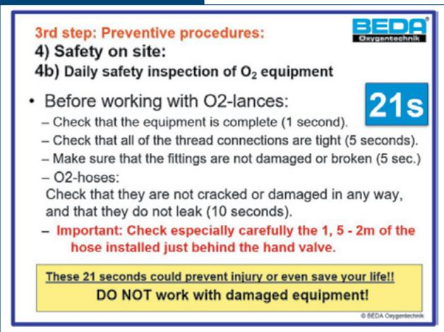
Example of an inspection sign posted at oxygen lancing locations at Steel Dynamics Inc.
