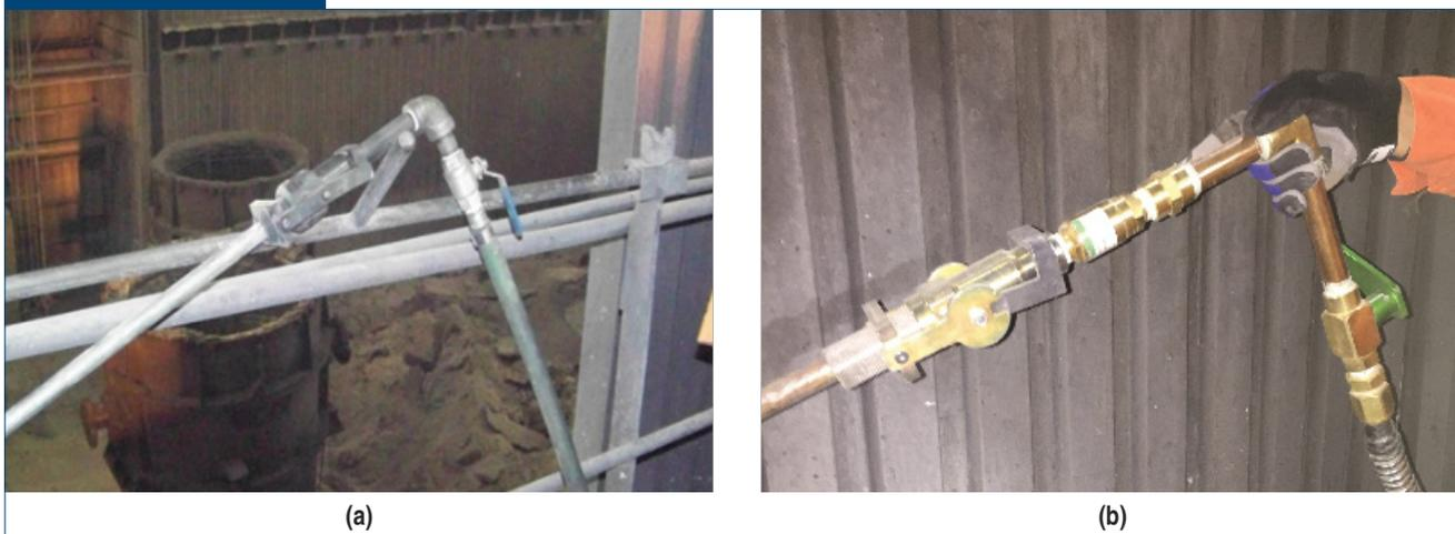
Pre-incident carbon steel oxygen lance setup (a) and post-incident improved setup (b).
