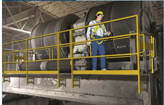
Conceptual fall protection solution for trolley maintenance.
