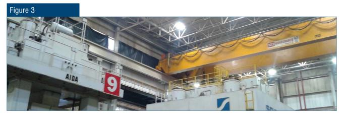
Overhead crane over a stamping press, which usually is made into a no-fly zone.
