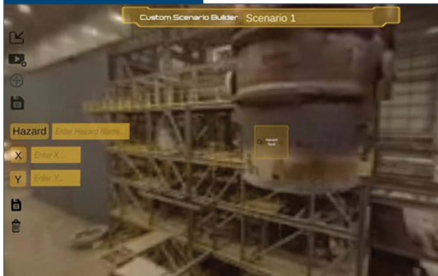
Overlays being displayed on top of a crane-suspended ladle.
