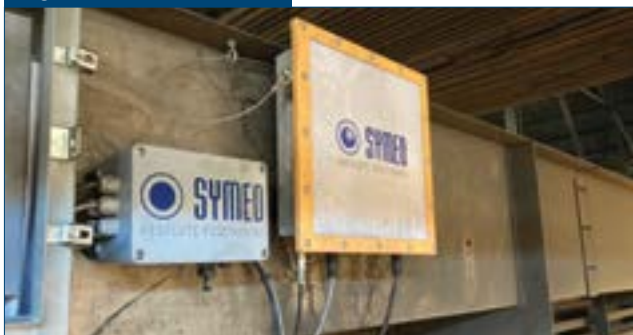
Radar sensor and the remote input/output device for the limit switch state, as mounted on a ladle crane.
