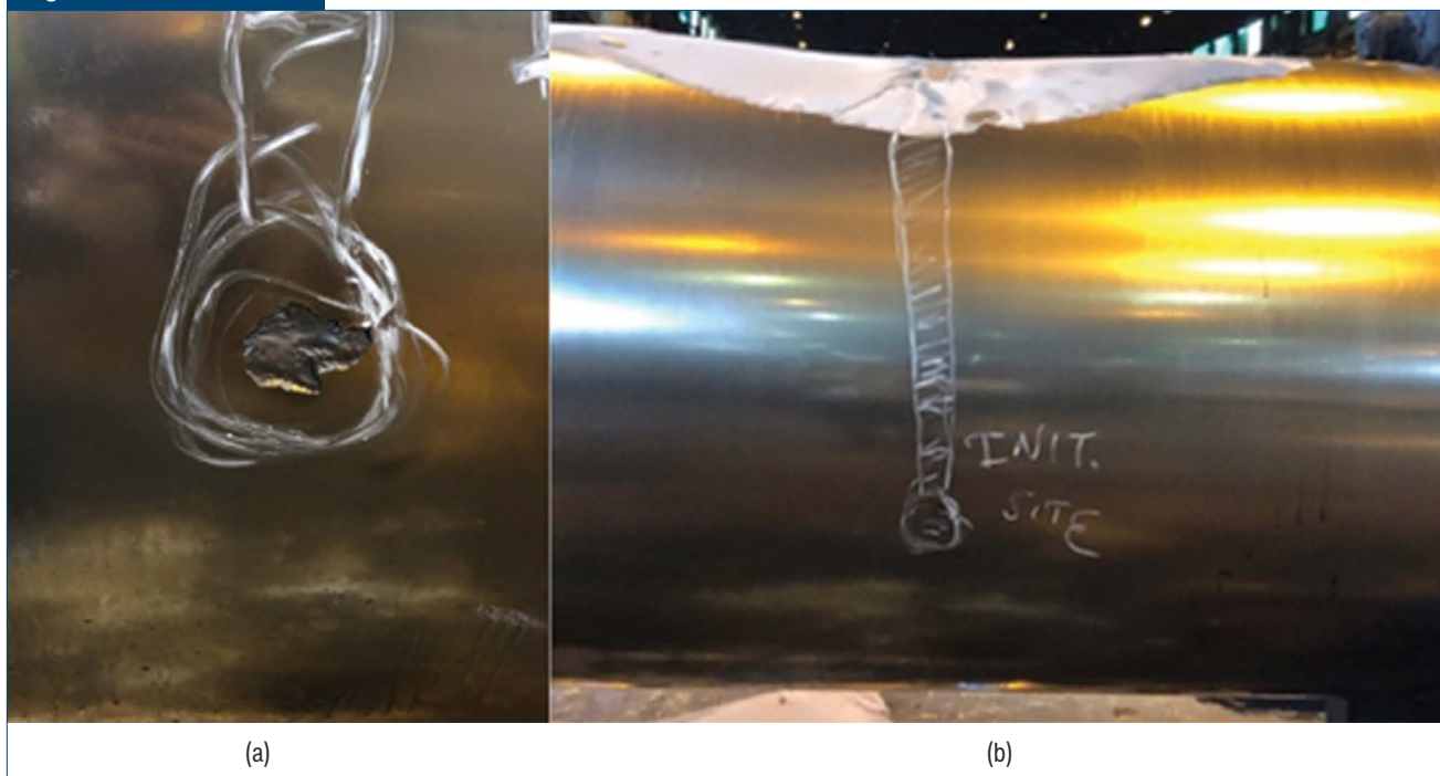
Surface damage caused by a high-stress mill accident (a) and stress conditions propagated a fracture band until explosive spalling of the roll barrel surface (b).
