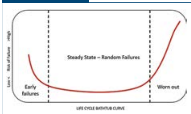
Life cycle of a system, illustrated in a bathtub curve.
