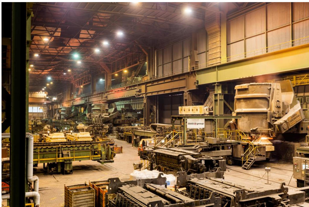
Turret of continuous caster No. 2. The four continuous casters at the Salzgitter Flachstahl plant were supplied by SMS group. Photo: Salzgitter Flachstahl
