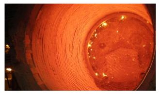
A staff of H steel stated, "This phenol free refractory brick reduces odor significantly without negative side-effect including heat resistance and wear resistances in comparison to traditional resin-bonded refractory product." He added, "We started this project 3 years ago as there were few complaints over odor and growing demand on the better workplace for site workers including crane drivers as most of gas goes up in the air. Finally this issue has been resolved successfully."
