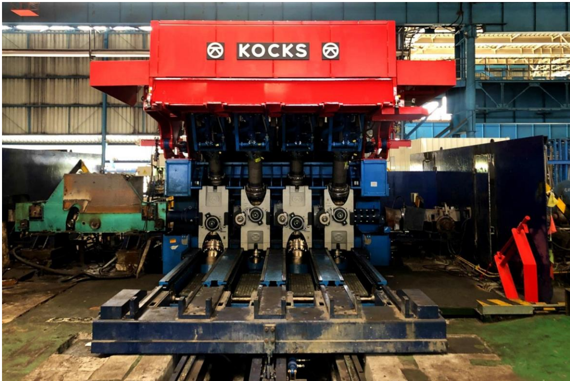
Caption: The commissioned RSB® 370++/4 is producing bar in coil and straight bars
