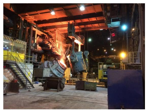
Primetals Technologies revamped the process optimization and the process control systems as well as the trunnion ring and tilting drive of an AOD converter of Valbruna in Italy.
