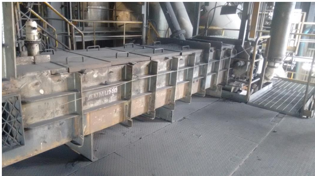
1998: AUMUND Drag Chain Conveyor, type LOUISE TKF, in ArcelorMittal's João Monlevade plant in Brazil (photo AUMUND)
