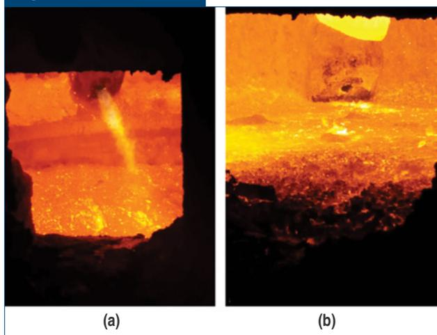
Injection angle (a) and close-to-steel/slag surface injector location (b).
