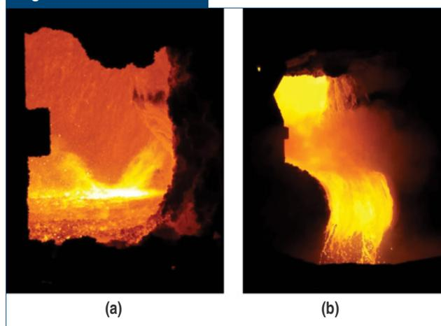
Example of very hard (after steel decarburization) (a) and very liquid (after slag reduction) (b) high-chromium slags.
