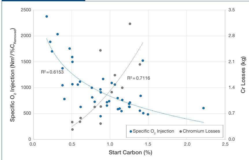
Specific O<sub>2</sub> injection rates and chromium losses with respect to initial carbon in steel.
