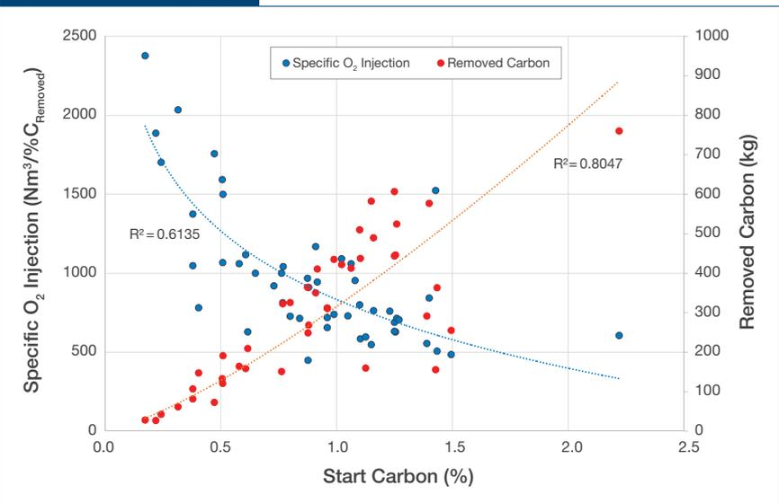
Specific O<sub>2</sub> injection and removed carbon referred to initial carbon in steel.
