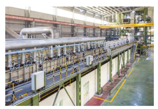
The new line will enable Ruifeng to coat 350,000 tons per year of cold strip for the construction and home appliances industries. The layer to be applied will be aluminum-zinc or zinc.
