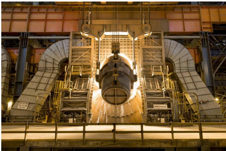
SMS group BOF converter, equipped with the maintenance-free lamella converter suspension system.
