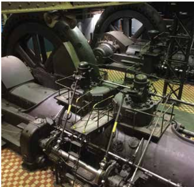
Fig. 2a: Gas-blowing engines.
