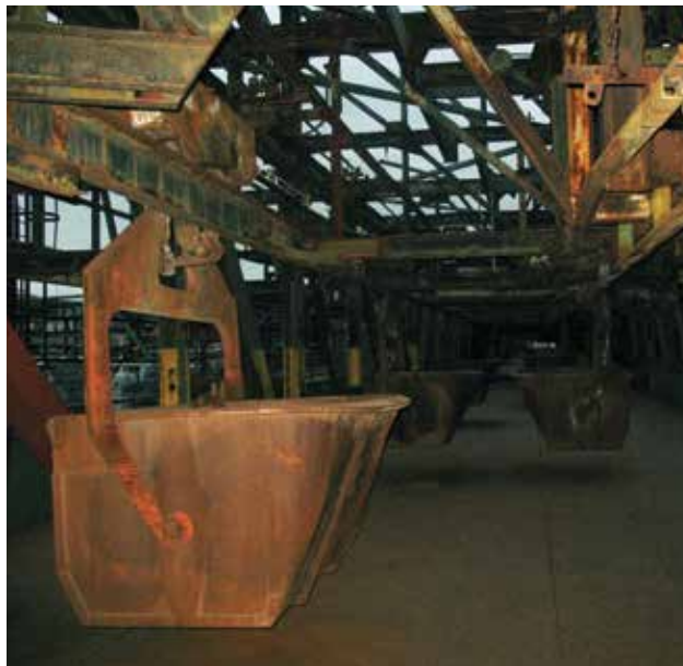
Fig. 2b: Suspended conveyer system.
