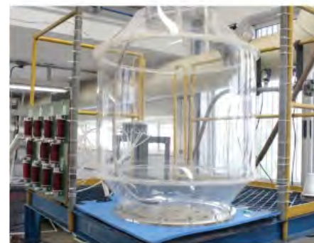
LaSiP plexiglas converter (scale 1:10)
