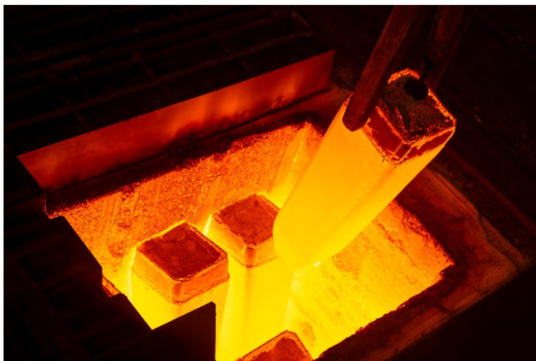
Figure 6. Photograph from current full scale operation reheating with 100% hydrogen as a fuel.
