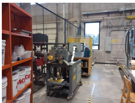
Figure 23. I&S Lab equipment, including a low intensity magnetic separator, briquetter, reduction under load test set up, reduction under load furnace reactors, high temperature high-capacity thermogravimetric analysis furnace, and a 7.5 kg induction furnace
