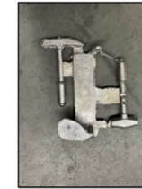
Casting with gating system
