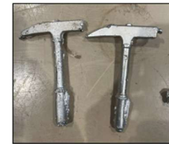
Aluminum green sand casting (left) compared to Petrobond (Right)
