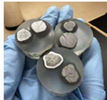
Figure 2: Mounted and sectioned DRI samples. Two to three DRI pieces were mounted in each sample.
