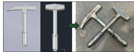
1 st Design Iteration to final Cast Bronze Product
