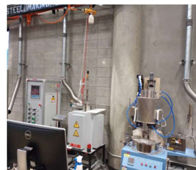
Figure 23. I&S Lab equipment, including a low intensity magnetic separator, briquetter, reduction under load test set up, reduction under load furnace reactors, high temperature high-capacity thermogravimetric analysis furnace, and a 7.5 kg induction furnace
