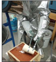
Casting Aluminum in Petrobond
