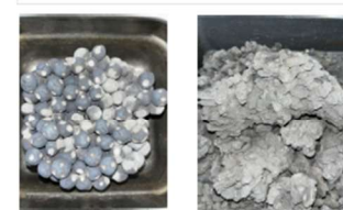
Figure (left): Reduced standard pellets from sticking and clustering index test (ISO 11256). The pellets retained their form throughout the reduction process.
