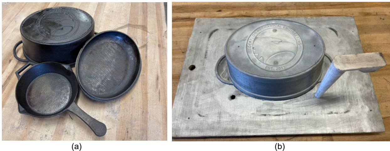
Figure 2. The finished cast iron cookware (a) and an example of the pattern made by the students (b)
