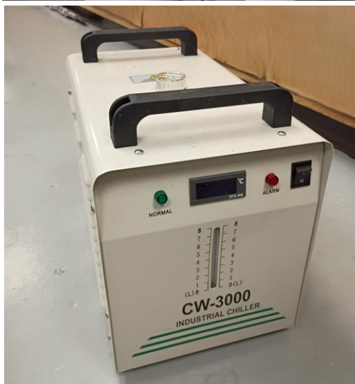
Figure 2. Equipment that was acquired to build “Forging-in-the-box” tool (a) Induction gun, (b) Metallic table, (c) bench vise, (c) Thermal camera, (e) water-cooled induction coil, and (f) compact chiller unit.
