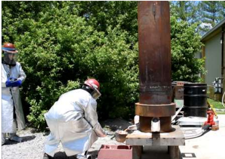
Figure 3. Iron melting cupola (12" inside diameter).
