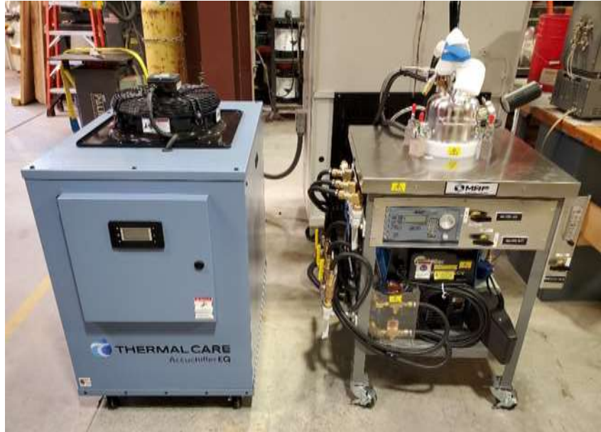
Figure 2. Vacuum/inert atmosphere, arc button melting (arc temperature up to 3500°C).
