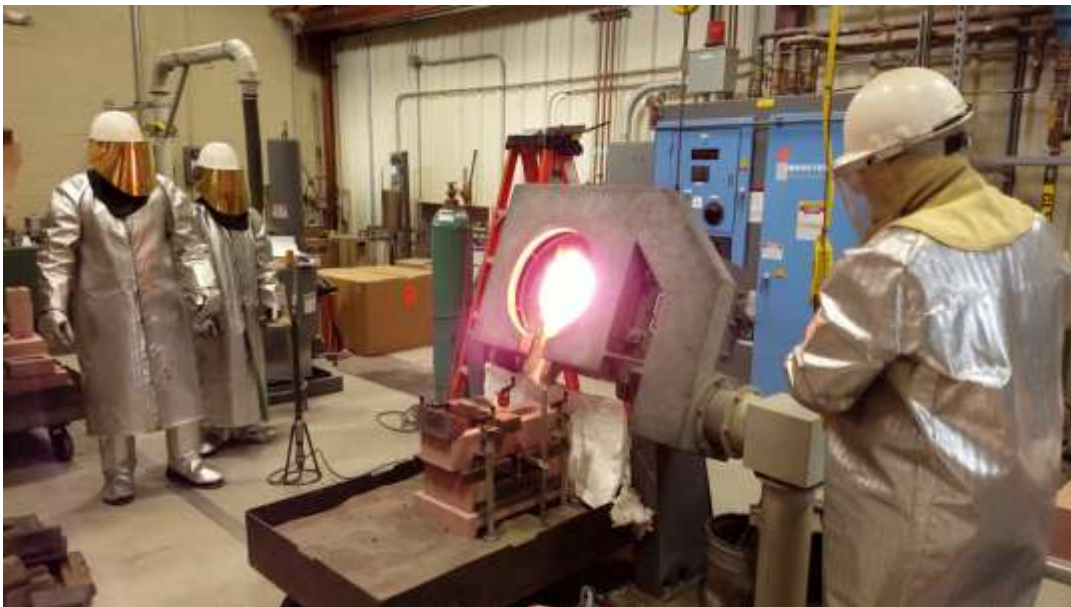
Figure 1. Induction melting furnace (300 lb capacity) pouring steel directly into a mold.
