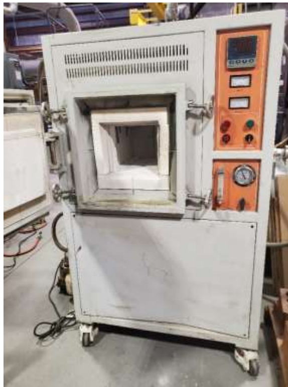
Figure 5. 1700°C, controlled atmosphere furnace recently donated by Nucor-Hertford.
