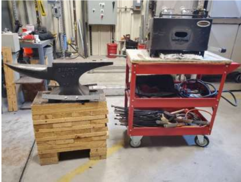
Figure 4. Propane forge and anvil used in Bladesmithing class to teach steel forging.
