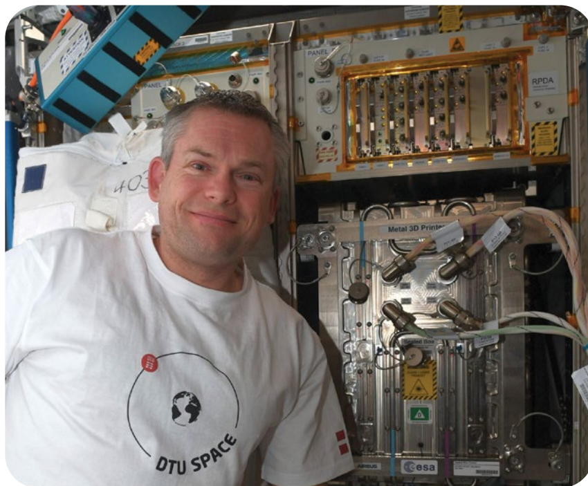
European Space Agency astronaut Andreas Mogensen installs the printer that enables 3D steel printing on the ISS. Photo courtesy of European Space Agency.
