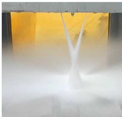
Figure 5. Two descaling nozzles spray water on a cold surface – cross spray -50mm on the left and comparison of a heat transfer coefficient for all experiments with opposite descaling on the right
