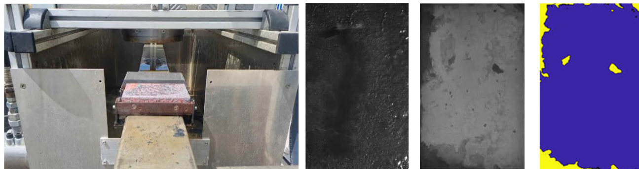
Figure 17. Experimental sample before descaling (on the left) and pictures of a plate surface from a descaling trial (from left to right): plate surface before descaling, plate surface after descaling and visualized descaled area (blue color)
