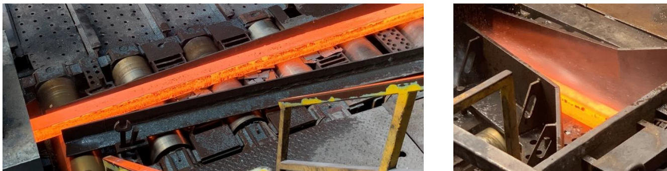
Figure 19. The left picture shows a bloom before descaling (very adhesive scales) and the right picture shows the bloom descaled by HIDROD
