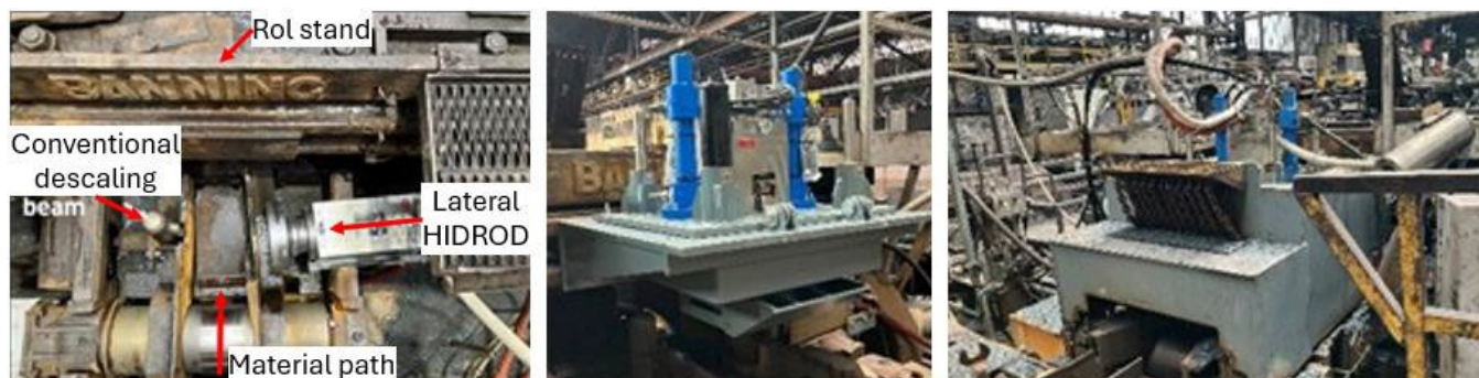
Figure 18. HIDORD installation on a blooming line – lateral installation (on the left), vertical installation (in the middle) and complete installation view with housing on the right
