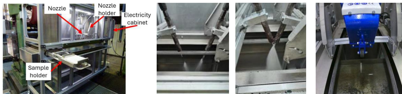
Figure 10. CRM pilot descaler (on the left), two nozzles mounted on the descaler and spraying oppositely (in the center) and shot blasting unit mounded on the descaler (on the right)
