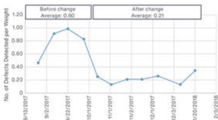
Changes in defect occurrence rate due to changes in mold vibration settings.
