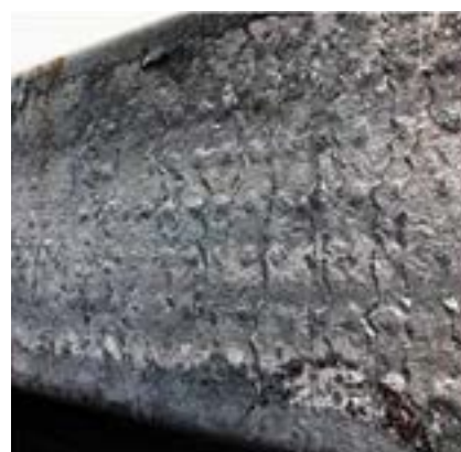
Cast piece with dimple marks remaining on the surface.
