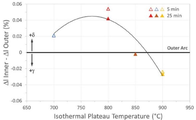
would not be significant, as the temperature differences are smaller, and the transformation of ferrite into austenite occurs at a slower rate. In this approach, the transformation from ferrite to austenite would be more uniform, as the cooling rate would be consistent. This would help eliminate distortion and spring effects, ensuring a comparable distribution of each phase in both the outer and inner arcs. This approach was field tested at SMS group Brazil yielding positive results.
