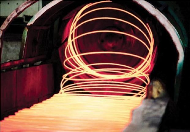
ensure product geometry, laboratory and field analyses at SMS group Brazil were conducted and successfully applied to the duplex stainless steel laying head pipe.
