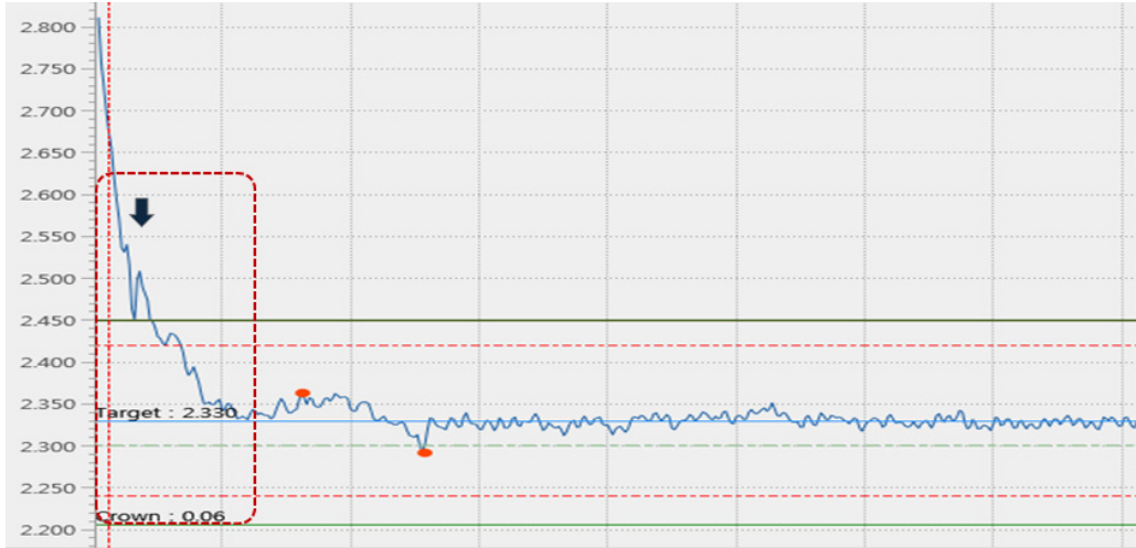
Fig. 1. Thickness profile at the head end of a low-carbon steel strip.
