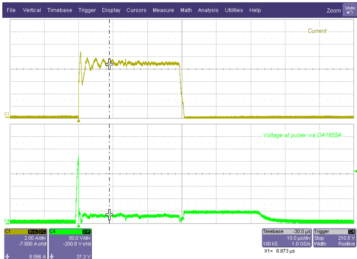
Fig. 1: Closed-loop current waveform with changing spark gap impedance. x-axis is time (10 \mu s/div); y-axes are (top) current (2A/div) and (bottom) voltage (50V/div).
