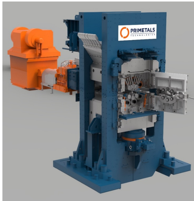
Figure 9: Advanced split-housing 20-high HZ-Mill
