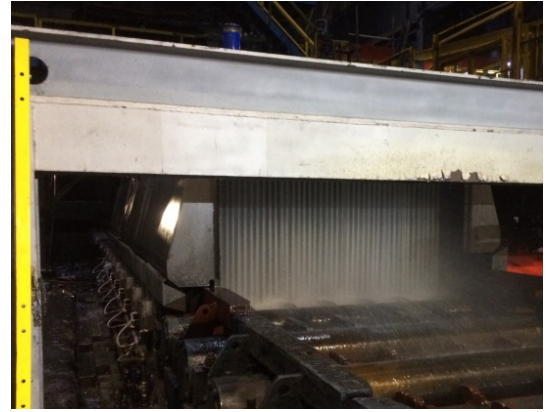
Figure 15. Homogeneous and effective water application of transfer bar cooling system.
