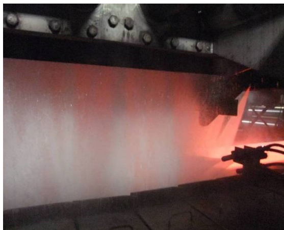
Figure 12. Power Cooling machine with cross sprays.
