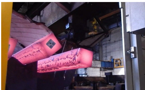
Figure 1: Billet tag application and reading
