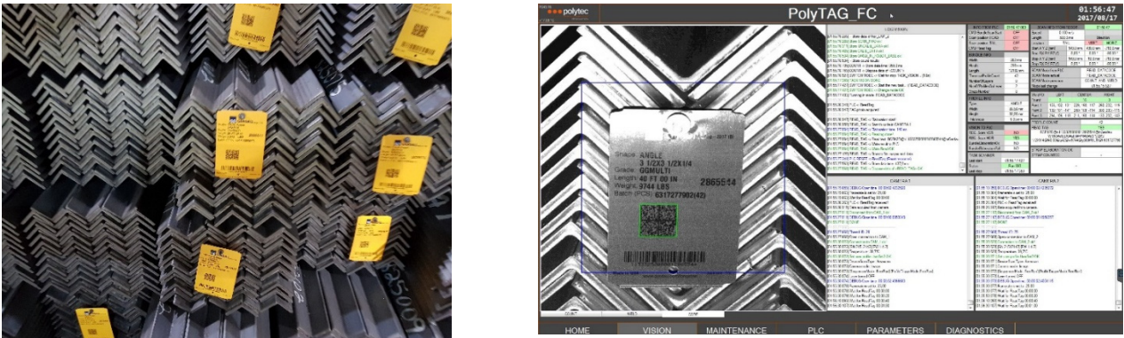
Figure 2: Bundle bars tagging robot and scan with point identification, piece counting and tag reading after welding
